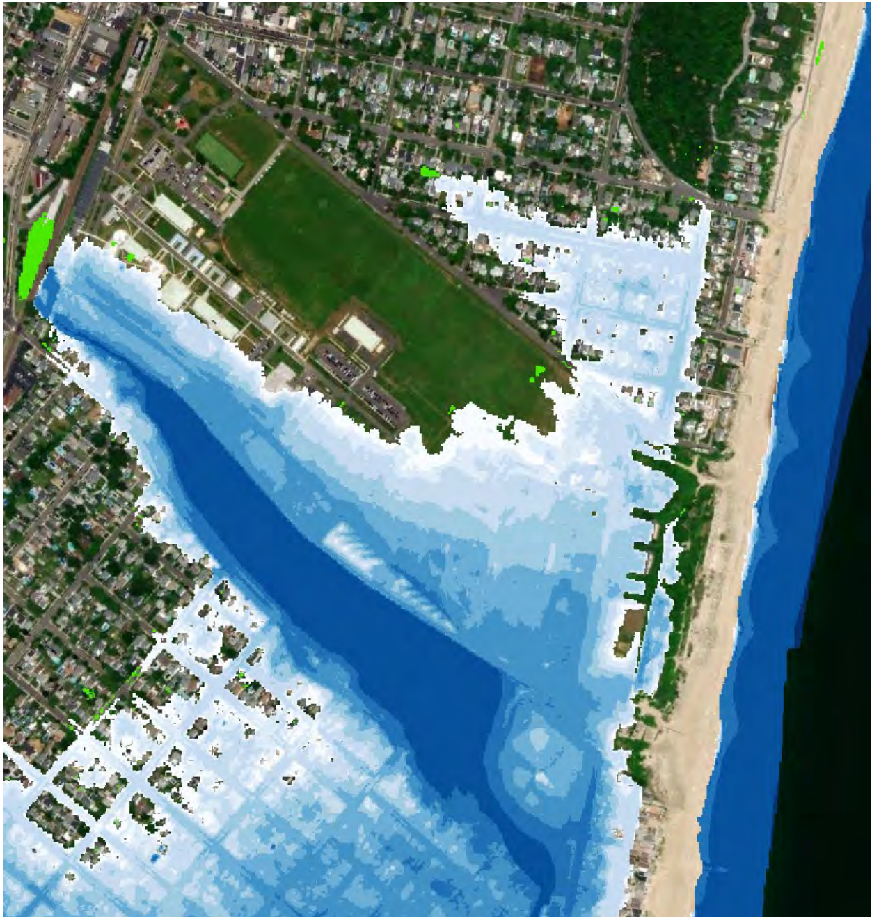
Figure 7. Sea Girt National Guard Training Center with a Total Water Level of 7 ft.
